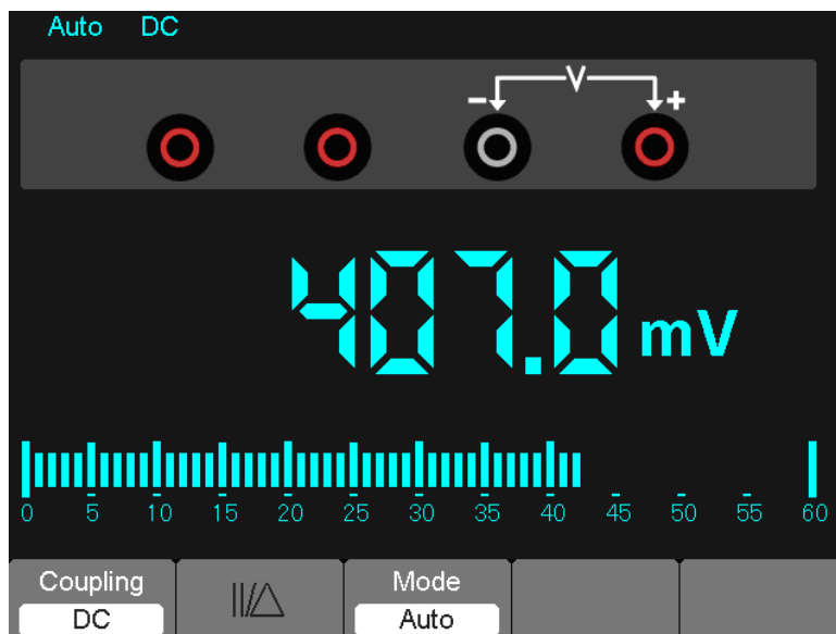
Figure 7-6 DC voltage Measurement
