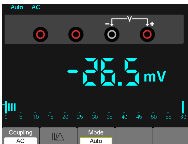
Figure 7-7 AC voltage Measurement
