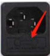
3. Remove the broken fuse and install a new one;
